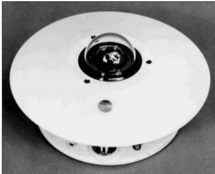
The Model 394 Pyranometer
