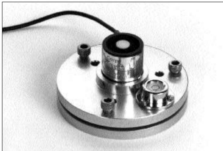
The Model 096 Pyranometer
