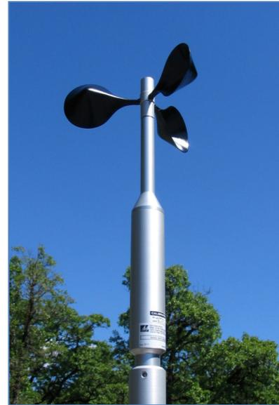
The design has been tested at three wind tunnels in the United States and the initial results suggest that the design meets "Class 1" performance requirements under IEC 61400-12-1 for the horizontal component of wind speed. Full classification testing is currently underway at Deutsche WindGuard. Results are expected by the end of calendar year 2011.
